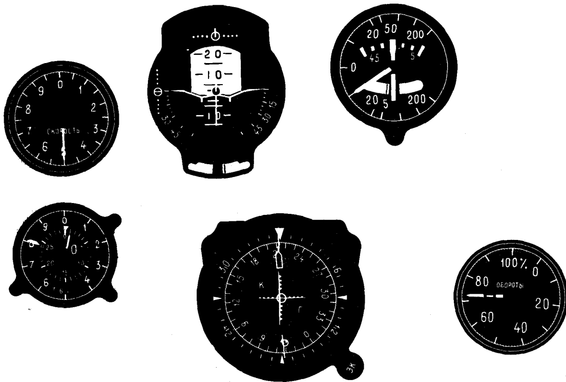
FIG. 72. INSTRUMENT READINGS CORRESPONDING TO GLIDESLOPE DESCENT FROM ALTITUDE OF 1000 m TO 600 m WITH LANDING GEAR EXTENDED
