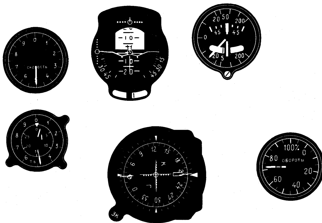
FIG. 71. INSTRUMENT READINGS CORRESPONDING TO GLIDESLOPE DESCENT FROM ALTITUDE OF 2000 m TO 1000 m WITH LANDING GEAR EXTENDED
